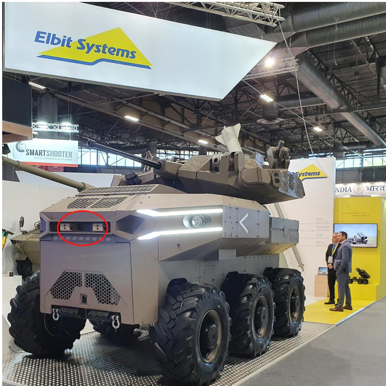
Integration of Foresight's QuadSight® software with Elbit's visible-light and thermal cameras
